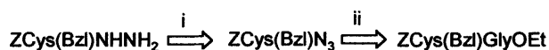
Scheme 4 Honzl-Rudinger azide coupling. Stages: i, HCl-anhydrous THF-BuONO, -20^\circ\text{C} , then \text{Et}_2\text{O} extraction; ii, GlyOEt-EtOAc. 86% yield overall.
